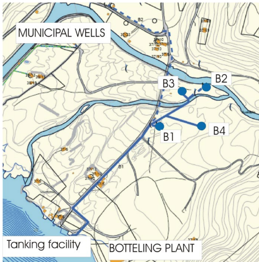
Municipal wells related to the water factory
